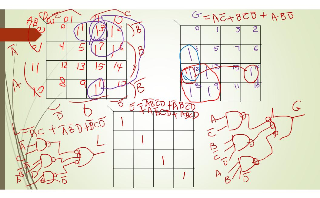
3. Design a circuit that can convert a BCD code into a Gray. a. Write the truth table for this circuit. b. Find the minimized logic equations in SOP and POS for each output c. Draw the corresponding all NAND and all NOR gates logic diagram for this circuit. Label all inputs and outputs.
